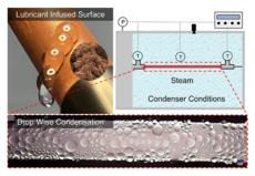
will be delineated. Focusing on application to power plant condensers, we will journey from the microstructure to the system level technoeconomic considerations to understand the extent of improvements in performance and levelized cost of condensers enabled by textured nonwetting surfaces.
