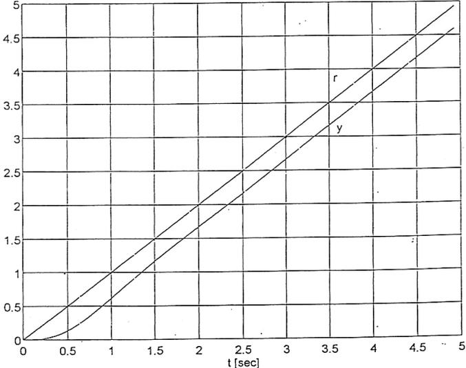
Figure 5: Closed-loop response of the system to a unit ramp input
