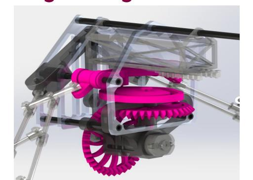
Active Folding with Bevel Gears and Cam and Carriage System
