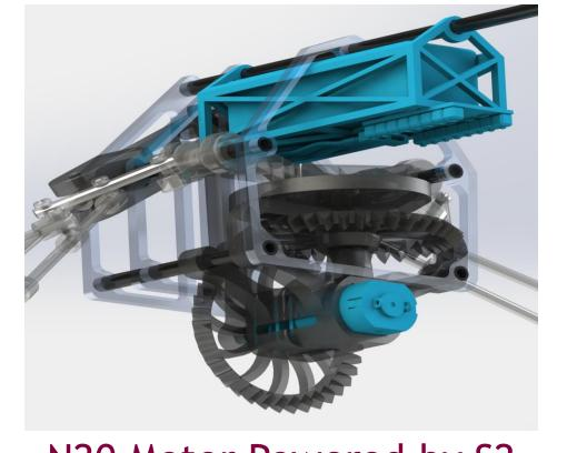
N20 Motor Powered by S2 Battery with Voltage Stepdown via buck converter
